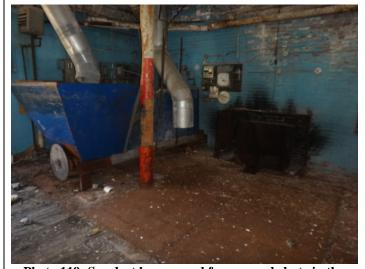
Photo 119: Sawdust hopper and former coal chute in the eastern portion of the second floor of the Site building.
