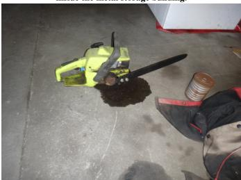
Photo 56: A leaking chainsaw observed inside the metal storage building.
