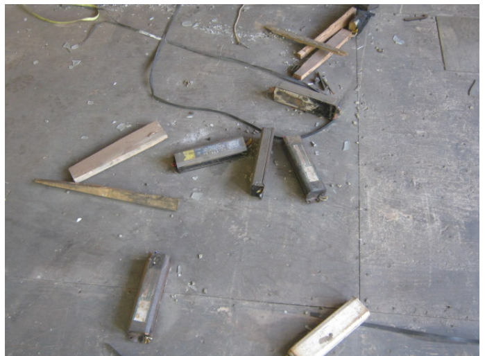
Presumed PCB-containing unlabeled electronic ballasts observed inside Main Mill Building.
